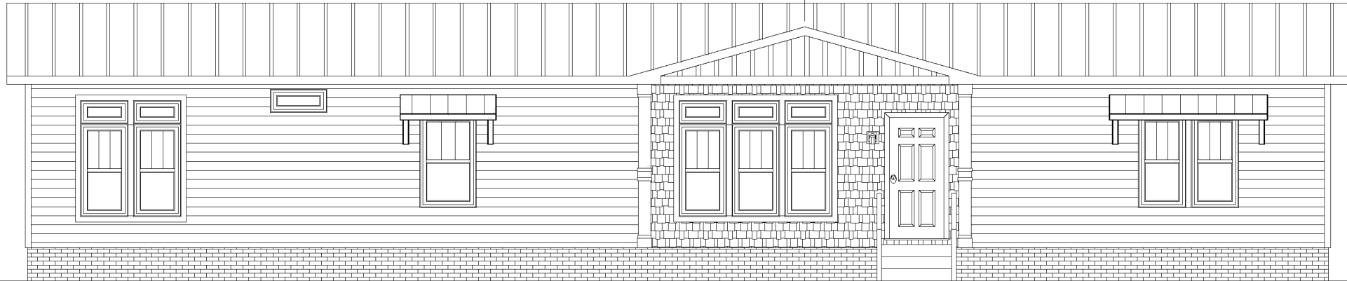
EZL32724B-32M507-METAL ROOF ELEVATION
